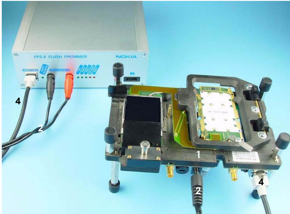
Figure 24: Module jig concept
